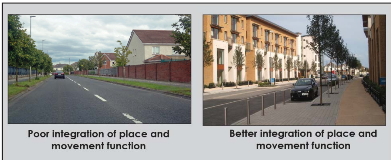
Figure 2.19: The most fundamental aspect of the creation of a sustainable street network is that designers clearly recognise that streets have both a place and movement function, so that streets are connected, enclosed, fronted onto and promote pedestrian and cyclist activity
