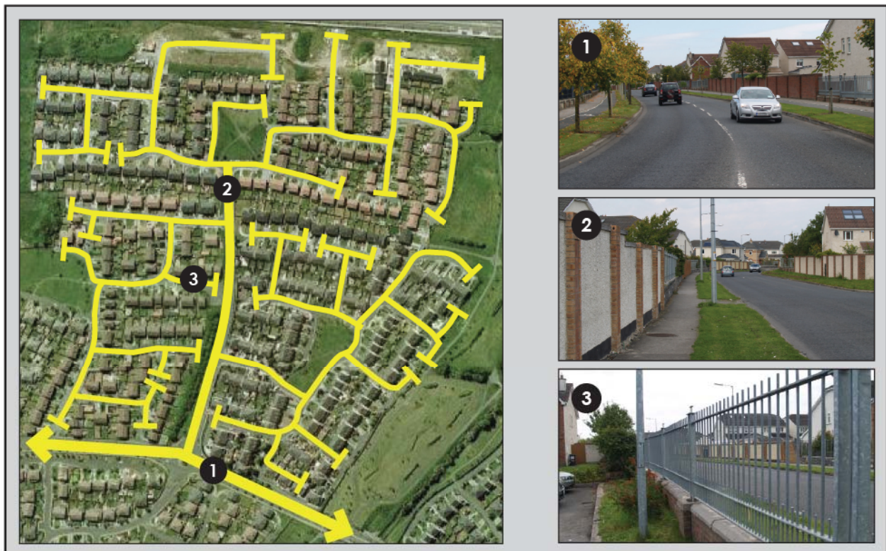
Figure 2.4: Example of a residential community designed according to the keynote principles of segregated street networks. 1) Distributor roads are designed to facilitate free flowing traffic and provide access to 2) neighbourhood cells. Movement through the cell enforced via a dendritic street layout of 3) cul-de-sacs that spread out like the branches of a tree (base image source: Google Maps).
