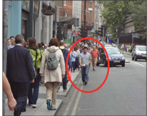
Figure 2.9: Footpath widths are inadequate, forcing pedestrians on to the carriageway, however, the width of the vehicular lane is in excess of what is generally required.
