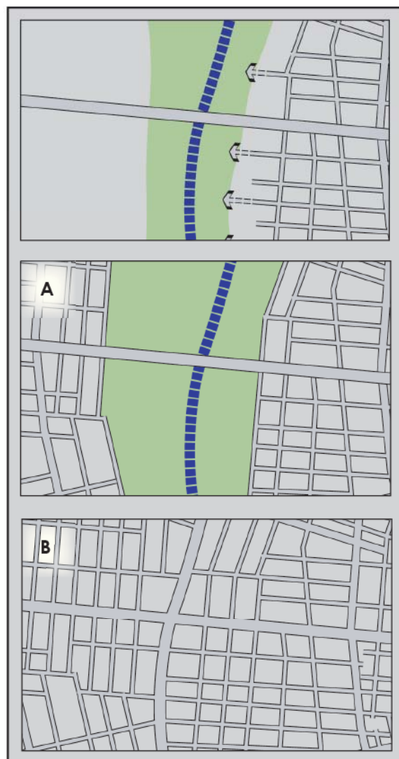
Figure 3.33: As urban expands toward an Urban Relief Road (top) a strategic decision will need to be made as to either maintain segregation and 'leapfrog' leaving a green belt (middle), or moderate speed, retrofit and integrate route (bottom).
