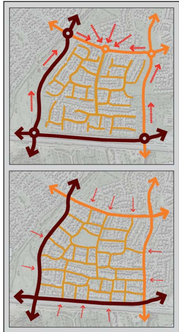
Figure 3.27: Highly segregated 'cell and distributor' networks channel faster moving traffic to large junctions where bottlenecks may occur (left). More permeable networks result in more frequent minor junctions with fewer vehicle movements (right) which calm traffic and are easier for pedestrians and cyclists to navigate.
