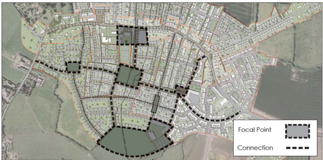
Figure 3.15: The Newcastle LAP (South Dublin County Council) illustrates how movement within the village is structured by connecting major Focal Points, which are also used to slow/discourage through traffic.
