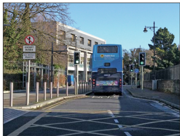
Figure 3.29: Example of a 'bus gate' in Tallaght, Co. Dublin, which filters permeability to allow for the free passage of buses whilst excluding other vehicles.
