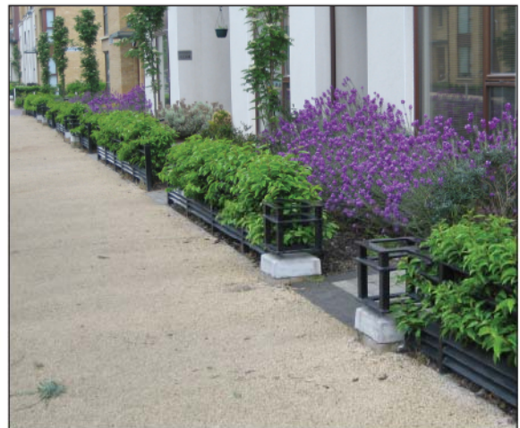
Figure 4.13: Privacy strip to the front of residential development. The strip provides a buffer and clearly define the private domain from the public.
