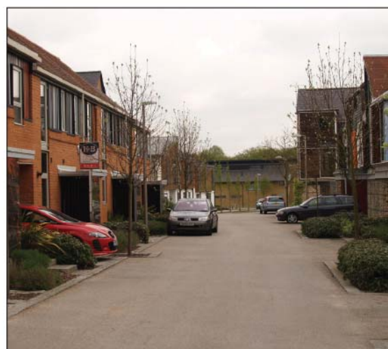
Figure 4.79. Example from New Hall, UK where a variety of in-curtilage and on-street parking is provided. On-street parking is provided semi-formally (indicated by the planting of trees). The parking of vehicles further calms traffic by providing a series of horizontal deflections.
