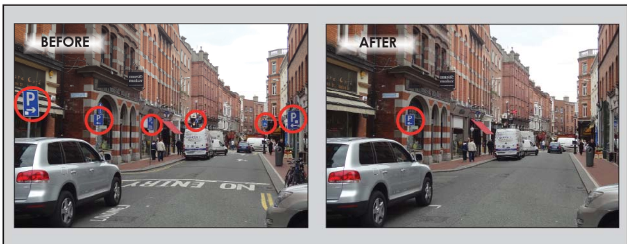
Figure 4.17: Example of the improvements to a streetscape that can be achieved where signage and line marking are substantially reduced. Note all changes have been made within the scope of the TSM.
