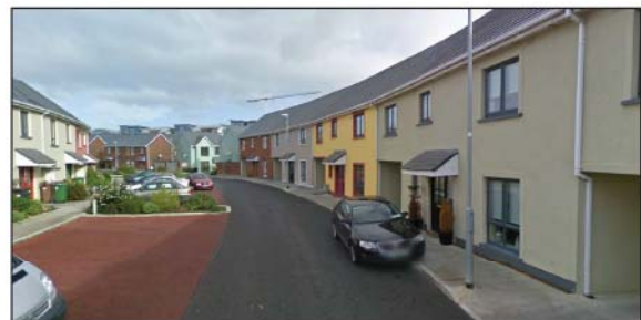
Figure 4.65: Example from Clongriffin, Co. Dublin where a change in the alignment of the street calms traffic as drivers proceed cautiously due to the uncertainty of what lay ahead (image source: Google Street View).
