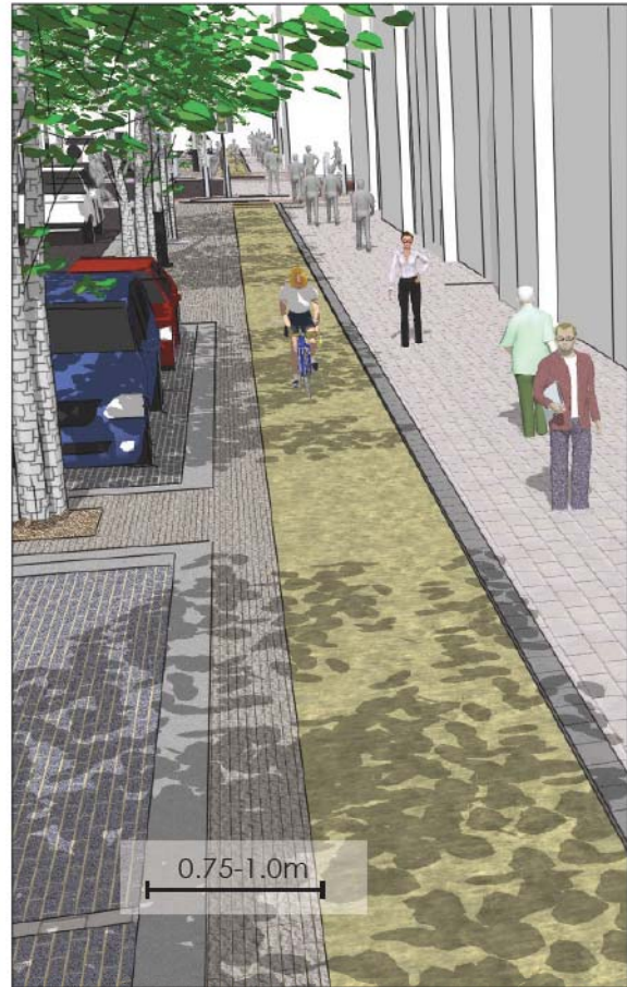
Figure 4.53: Example of a narrow verge between a cycle track and on-street parking. This verge provides a buffer that protects cyclists from opening doors.
