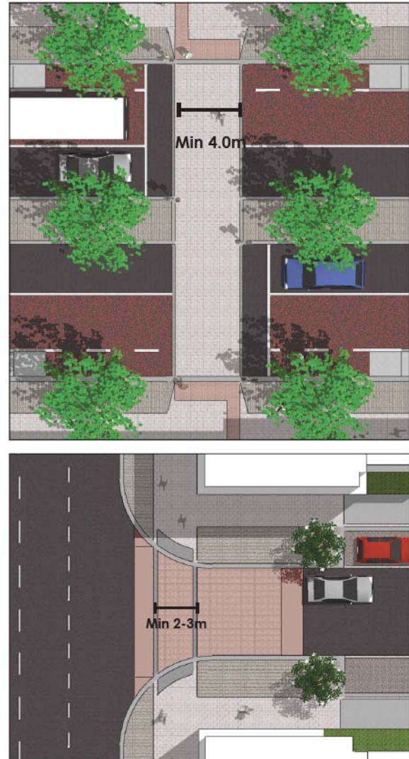
Figure 4.41: Standard crossing widths to be used in most circumstances across the main carriageway of Access or Link streets and across side junctions with Local streets.
