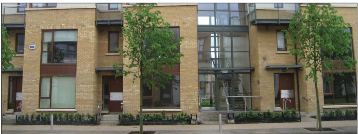
Figure 4.14: A fine grain residential environment where all ground floor dwellings are directly accessible from the street via 'own door' entrances. Note, in this instance access to upper floors is provided via internal lobby areas.
